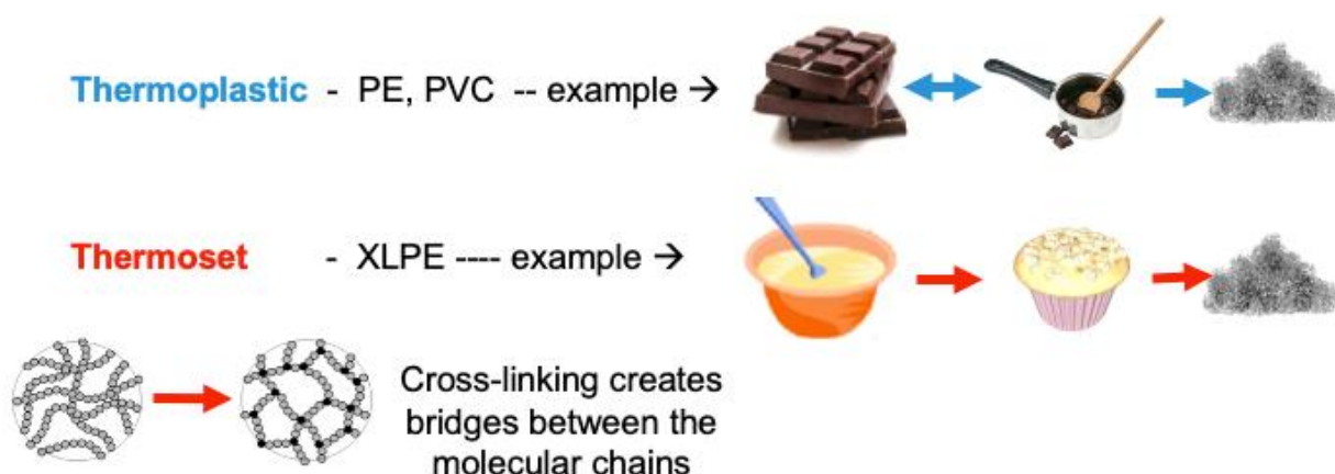
Figure 21 – The two most common insulation types
