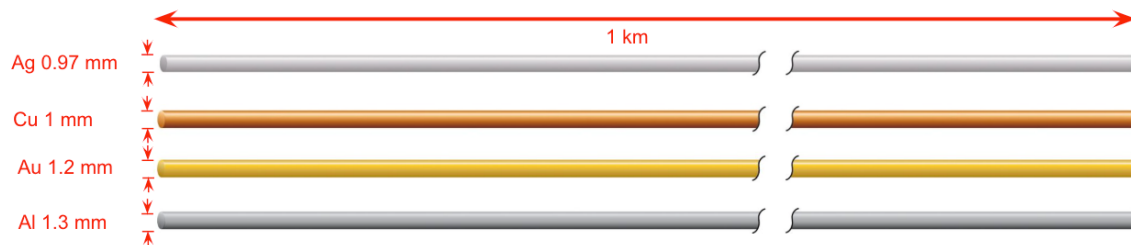
Figure 9 – The four best conductors electricity
